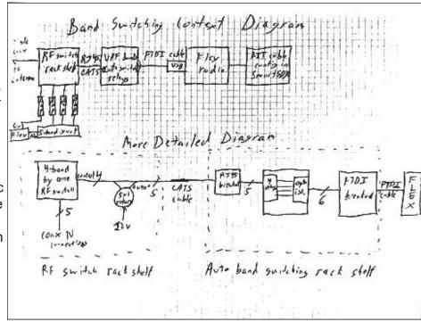
manual rotary switch) was intended to prevent conflict between manual and automatic band selection. The signals would be passed between the RF switching shelf and the future automatic selection shelf via a CAT-5 cable.
