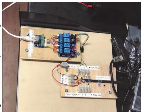
relay, I could use 4 signal relays to drive the RF relay. Using a new BIT cable would require configuring the cable in SmartSDR to activate a bit wire for each of the four VHF bands, with due attention to configuring active low or active high FTDI output bits (turns out I needed active low bits, see below).
